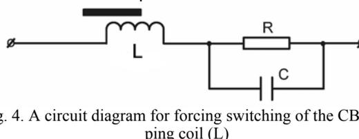
Fig. 4. A circuit diagram for forcing switching of the CB tripping coil (L)
