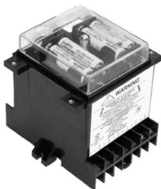
Fig. 1. One of the modern capacitor trip unit providing accumulation and long storage of energy for a feed of trip coil of circuit breaker at absence of an auxiliary voltage
