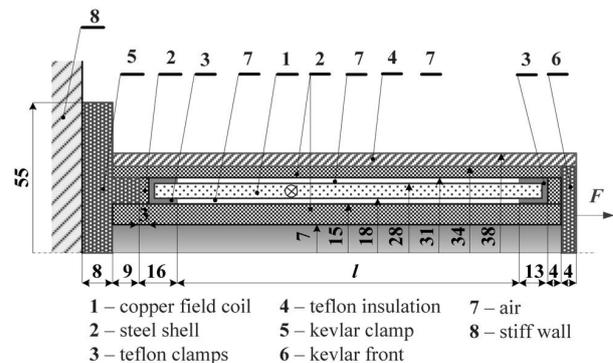
Fig. 4. Arrangement of a thermoelastic actuator [25]
