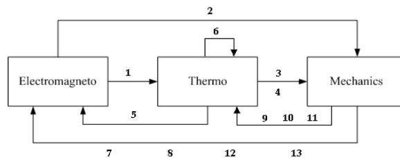
Fig. 1. Main "physical domains" of multi-physical simulations and their interactions
