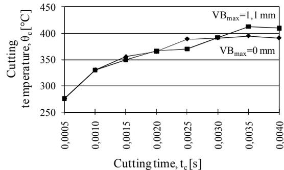
Figure 5 – Cutting temperature diagram by finite element modeling
