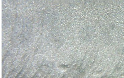
Figure 1 – Characteristic Surface of Aluminium Alloy Cut by Abrasive Waterjet
