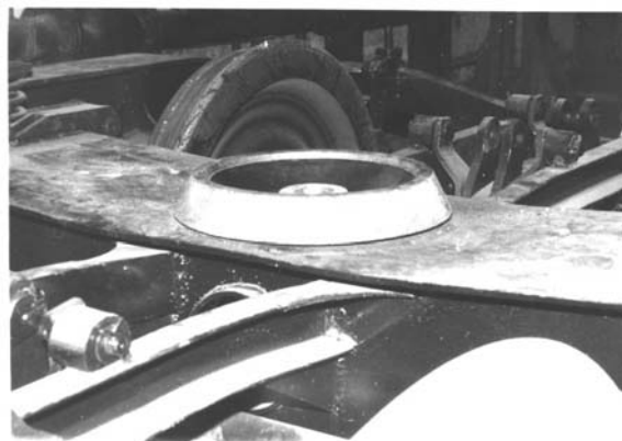
Figure 4 – Moment from the assembly of the force transducer in the king-pin bearing beam
