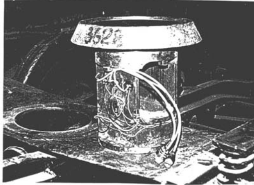
Figure 2 – Force transducer for three orthogonal directions
