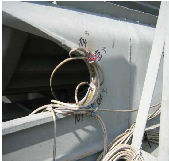
Figure 8 – Studied stress concentrator area
