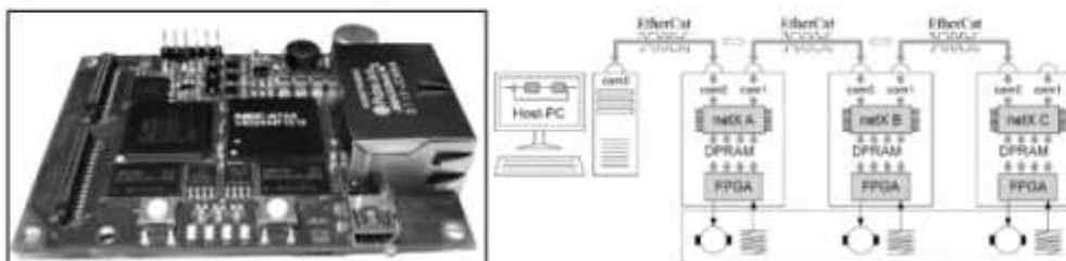
Figure 2. Flexible communication system based on netX processors.
