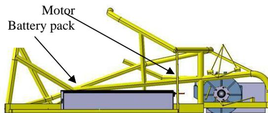
Figure 2: CAD model of the front part according to first stage.
