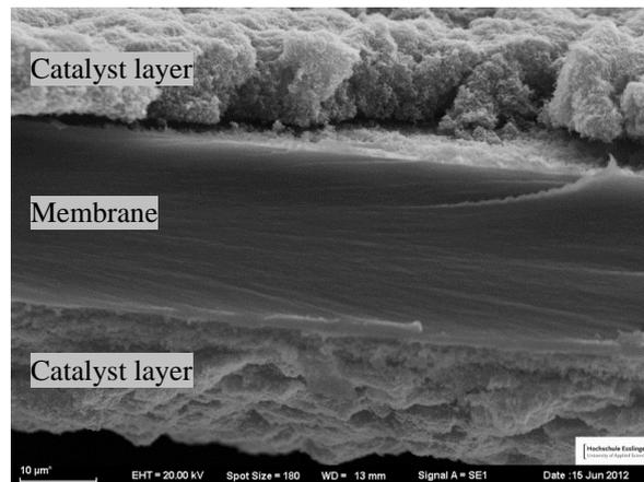
Figure 3: SEM cross-section picture of a CCM using spraying method.
