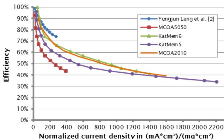
Figure 4: Efficiency curves normalized to the catalyst loading of produced MEAs in comparison to [2].
