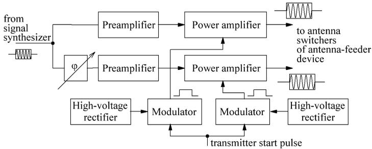
Fig. 4 – Block diagram of the IS radar transmitter
