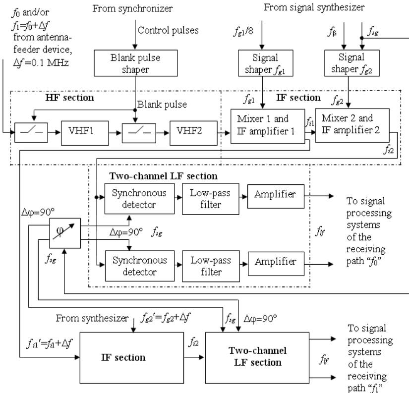
Fig. 5 – Block diagram of the IS radar receiver
