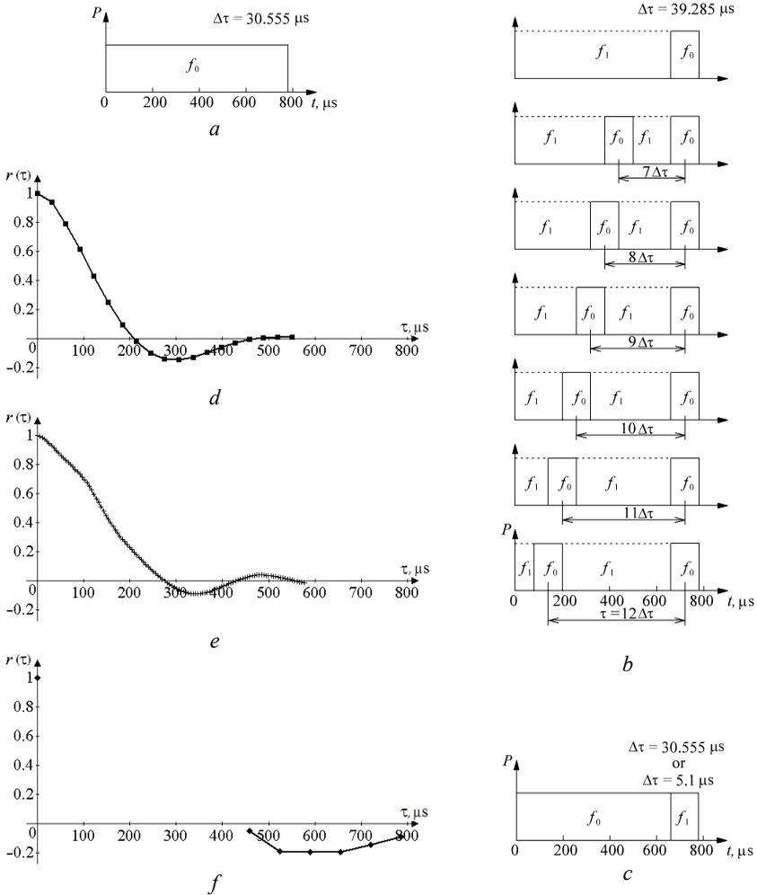
Fig. 7 – Diagrams of sounding signal for three main modes of Kharkiv IS radar: *a* – one-pulse mode, *b* – double-pulses mode, *c* – dual frequency sounding with long and short radio pulses. IS signal ACFs: *d* – lag step  $\Delta\tau$  equals 30.555  $\mu\text{s}$ , *e* – 5.1  $\mu\text{s}$ , and *f* – 39.285  $\mu\text{s}$ .
