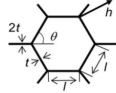
Here  $t$  is the thickness of the hexagonal cell wall,  $l$  is the dimension of the cell,  $\theta$  is inclination angel,  $\rho_0$ ,  $E_0$  and  $G_0$  are the density, Young's modulus and shearing modulus, respectively, of foil material of which the honeycomb core is made.  $\rho_{eff}$  is the effective mass density of the honeycomb material.
