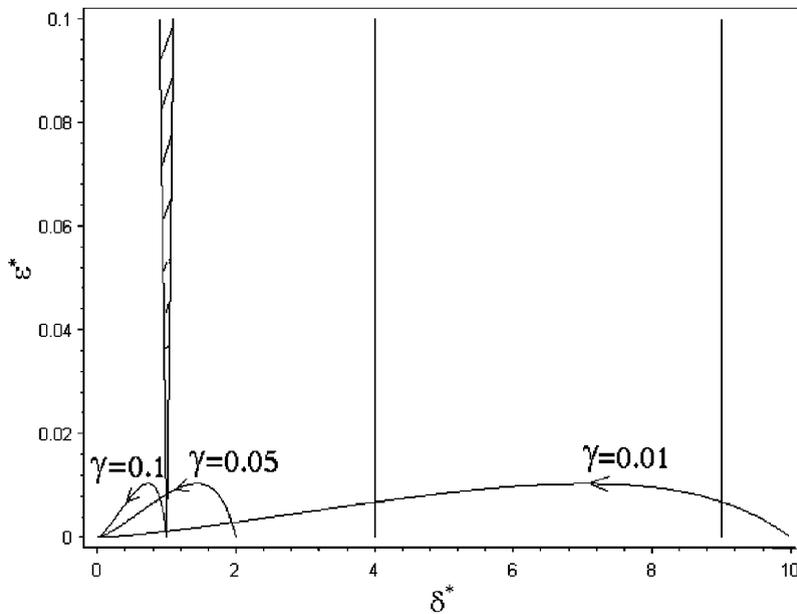
Fig. 3. Regions of instability of the localized mode (for some fixed values of the parameter  $\gamma$ ) in a plane of the Mathieu equation parameters when the amplitude  $X_0$  increases. Direction of the vibration amplitudes increase is shown by pointers.
