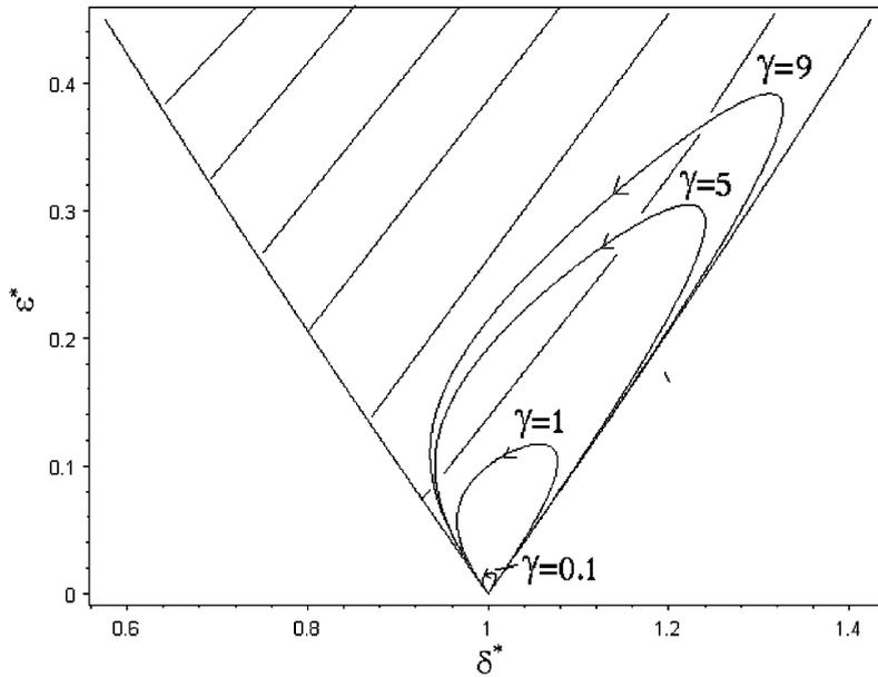
Fig. 2. Region of instability of the non-localized mode (for some fixed values of the parameter  $\gamma$ ) in a plane of the Mathieu equation parameters when the amplitude  $X_0$  increases. Direction of the vibration amplitudes increase is shown by pointers.
