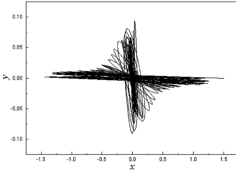
Fig. 8. Dynamics of system (1) with dissipation: transfer from the localized mode to non-localized one when the vibration amplitude decreases.
