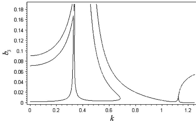
Fig. 14. Frequency response  $b_3(k)$  in system (26): two-harmonic approximation of the forced oscillations.
