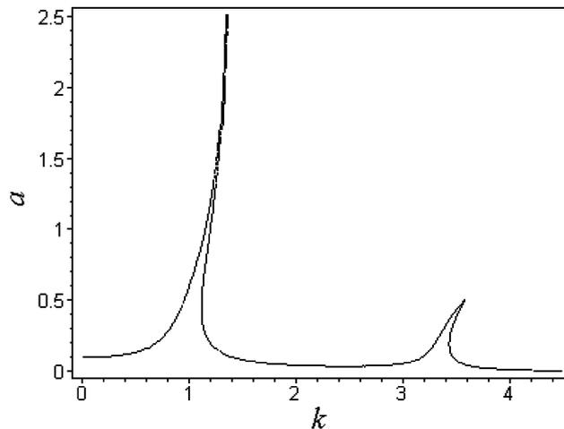
Fig. 9. Frequency response  $a(k)$  in system (27): damped forced oscillations.
