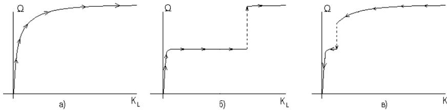
**Figure 4.** The engine frequency transfer. (a,c) the Zommerfeld effect is absent, (b) the Zommerfeld effect exists.
