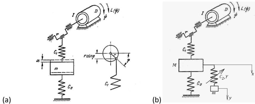
**Figure 1.** (a) The nonlinear system with limited power supply. (b) The non-ideal system with the nonlinear absorber
