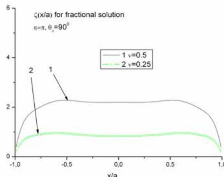
**Figure 2.** The ratio  $\zeta(x)$  for the fractional strip for  $\varepsilon = \pi$ ,  $\theta_0 = 90^\circ$ .
