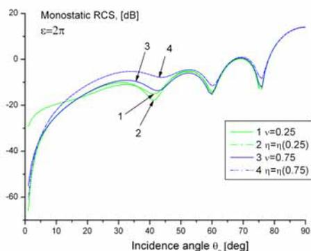
**Figure 1.** Monostatic RCS versus the incidence angle for  $\varepsilon = 2\pi$ . (1) fractional strip  $\nu = 0.25$ ; (2) impedance strip for  $\nu = 0.25$ ; (3)  $\nu = 0.75$ ; (4) impedance corresponding to  $\nu = 0.75$ .
