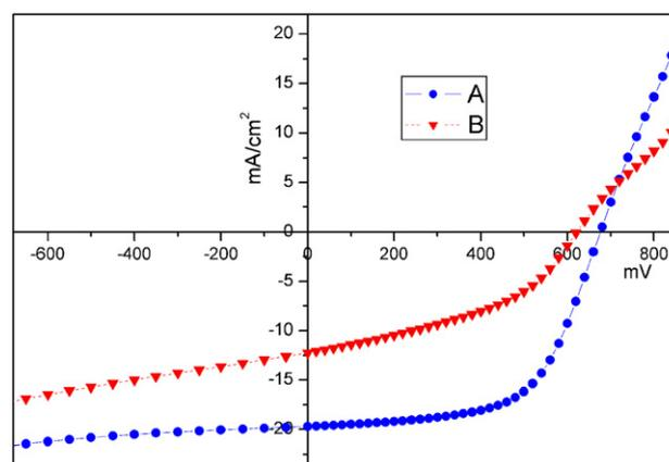
Fig. 3. Front (A) ( $V_{oc} = 676$  mV,  $J_{sc} = 19.7$  mA/cm<sup>2</sup>, FF = 60.5%,  $\eta = 8\%$ ) and back (B) illuminated ( $V_{oc} = 622$  mV,  $J_{sc} = 12.2$  mA/cm<sup>2</sup>, FF = 43%,  $\eta = 3.2\%$ ) CdTe solar cell with 1-μm-thick absorber.
