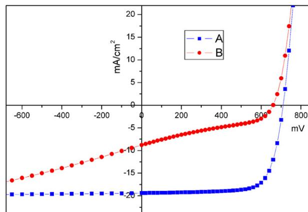
Fig. 2. Front (A) ( $V_{oc} = 710$  mV,  $J_{sc} = 19.4$  mA/cm<sup>2</sup>, FF = 74.6%,  $\eta = 10.3\%$ ) and back (B) illuminated ( $V_{oc} = 659$  mV,  $J_{sc} = 8.8$  mA/cm<sup>2</sup>, FF = 36%,  $\eta = 2.1\%$ ) CdTe solar cell with 2.5-μm-thick absorber.
