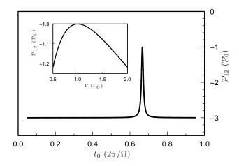
FIG. 2: Main: The noise  $\mathcal{P}_{12}$ , Eq. (2), as a function of the time  $t_0$  when an electron is excited out of the metallic contact by the voltage pulse  $V_2(t)$ . The plot assumes that the half-width of the voltage pulse at the MC and the pulse of the SES are the same ( $\Gamma = \Gamma_0$ ). The parameters of the SES, Eq. (A1), are:  $T = 0.1, U_0 = 0.25, U_1 = 0.5$ . Inset: The noise at the minimum as a function of  $\Gamma$ .
