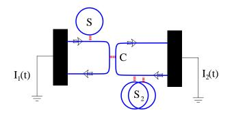
FIG. 5: (color online) A mesoscopic electron collider circuit with a single-electron source S and a two-particle source  $S_2$ . At the quantum point contact C the particles emitted by different sources can collide if the times of emission were adjusted properly. Solid blue lines are edge states with direction of movement indicated by arrows. Short dashed red lines are quantum point contacts connecting different parts of a circuit. Black rectangles are metallic contacts.
