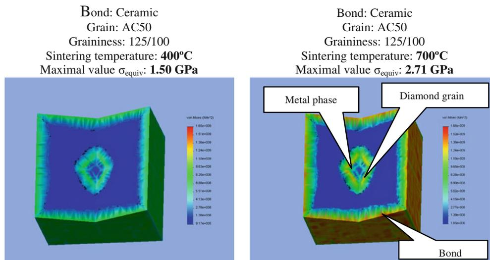
**Table 1** Maximum values of equivalent stress for various components of the system "bond-metal phase-grain" with diamond grain AC100 (200/160)
