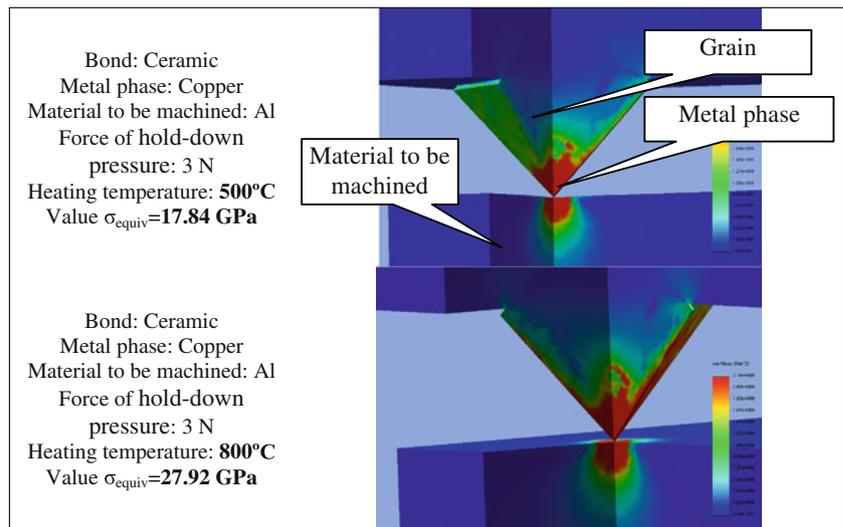
num, sodium-borosilicate glass) was studied and the positive influence of the coatings on diamond grain integrity retention at fabrication stage of diamond wheel is confirmed (Fig. 5). It is established that molybdenum coating of diamond grains is most effective to ensure retention of their integrity in the course of sintering of the diamond-bearing layer.
