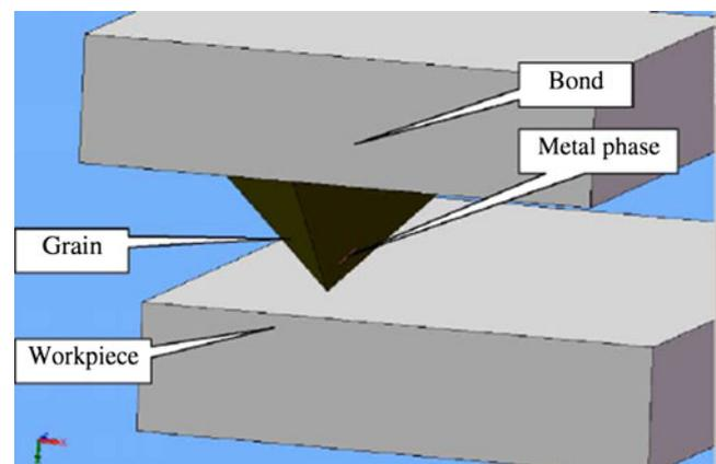
**Fig. 6** 3D model "bond-grain-metal phase-workpiece" with finite element mesh
