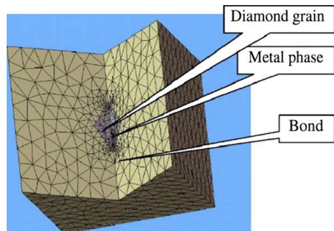
**Fig. 2** Generated finite-element mesh in 3D model
