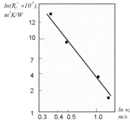
**Figure 1.** The comparison of velocity influence on asymptotic value of fouling thermal resistance predicted by equation (11) with experimental data of Karabelas et al, 1997.
