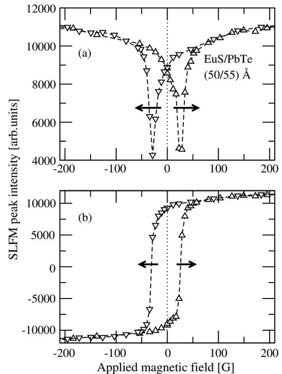
**Figure 6.** (a) The intensity of the first SL Bragg peak in sweeping applied magnetic field for EuS/PbTe (50/55) Å superlattice; (b) the intensity data converted to ferromagnetic hysteresis loop for this SL (see the text): no typical signature of the AFM IC is visible.
