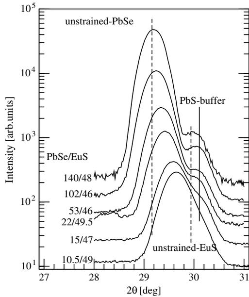
**Figure 7.** X-ray (200) reflection, measured in transmission geometry, from a number of pseudomorphic EuS/PbSe superlattices with approximately constant EuS and increasing PbSe layer thicknesses. Apart from the PbS buffer peak, there is only one maximum, which confirms the coincidence of the in-plane lattice parameters of EuS and PbSe. The value of the common in-plane lattice parameter shifts towards the unstrained (bulk) PbSe lattice constant as the thickness of the PbSe layer increases.
