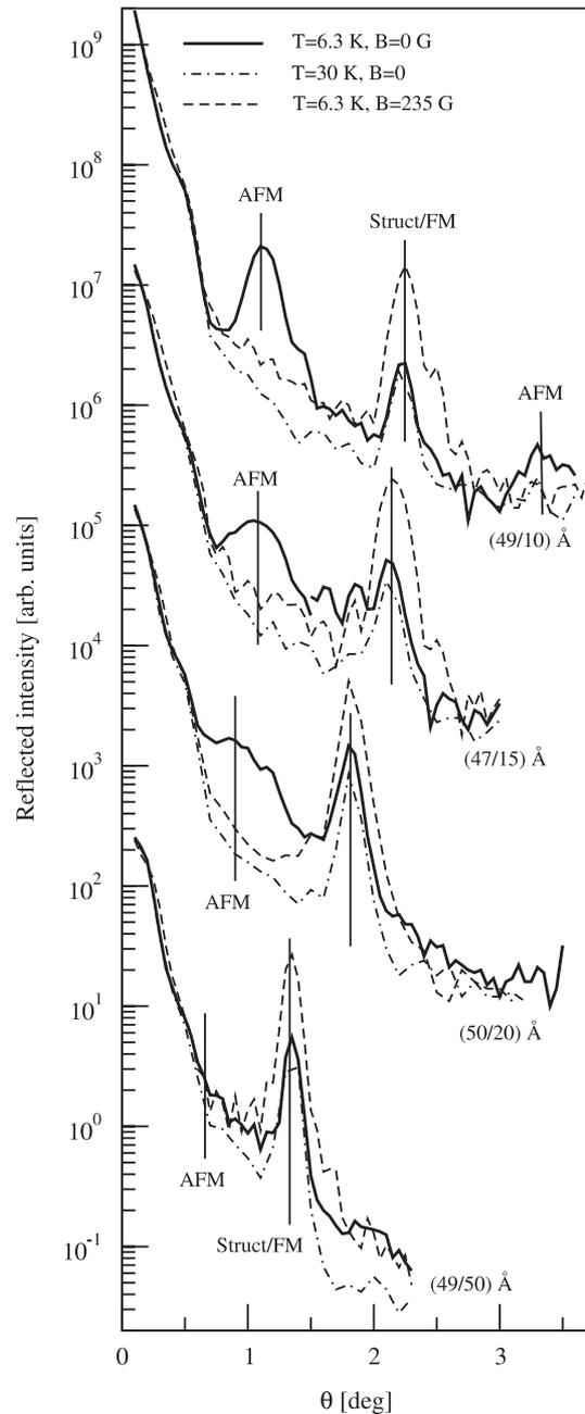
**Figure 2.** Unpolarized neutron reflectivity profiles for several EuS/PbSe superlattices with increasing thicknesses of the PbSe spacer. Data taken below (solid line) and above (dotted–dashed line) the EuS Curie point (16.6 K) and in zero and saturating, 235 G (dashed line) magnetic fields.
