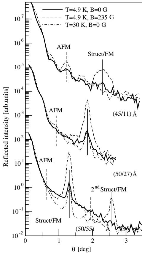
**Figure 5.** Unpolarized neutron reflectivity profiles taken below and above EuS Curie temperature ( $T_C = 16.6$  K) in zero and saturating (235 G) magnetic field for three EuS/PbTe samples with different thicknesses of the nonmagnetic spacer PbTe.
