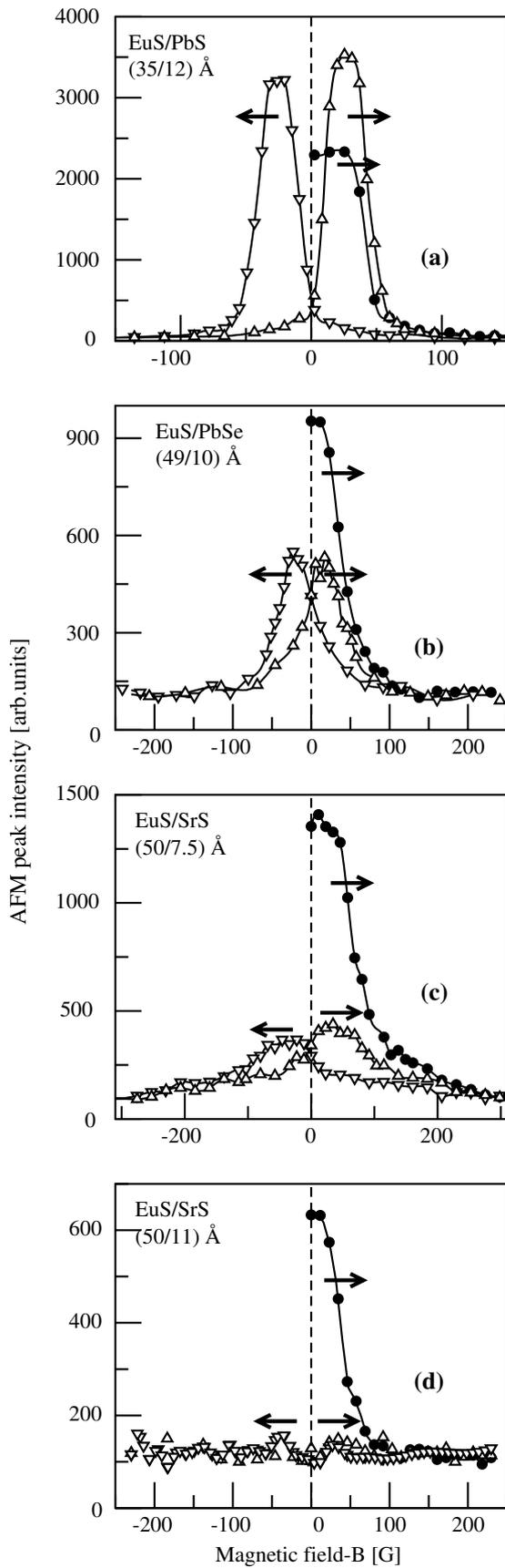
**Figure 3.** The intensity of the AFM SL Bragg peak versus sweeping magnetic field ('AFM hysteresis loops') for (a) EuS/PbS, (b) EuS/PbSe and (c), (d) EuS/SrS SLs. The direction of the field sweep is marked by the arrows.
