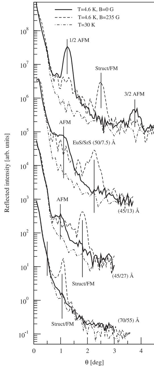
**Figure 1.** Unpolarized neutron reflectivity profiles for four EuS/SrS superlattices with increasing thicknesses of the SrS layer. Data taken below and above the bulk EuS Curie point (16.6 K), solid and dotted–dashed lines, respectively, and in zero and saturating (dashed line), 235 G, magnetic fields. The curves for different samples have been vertically translated for clarity.
