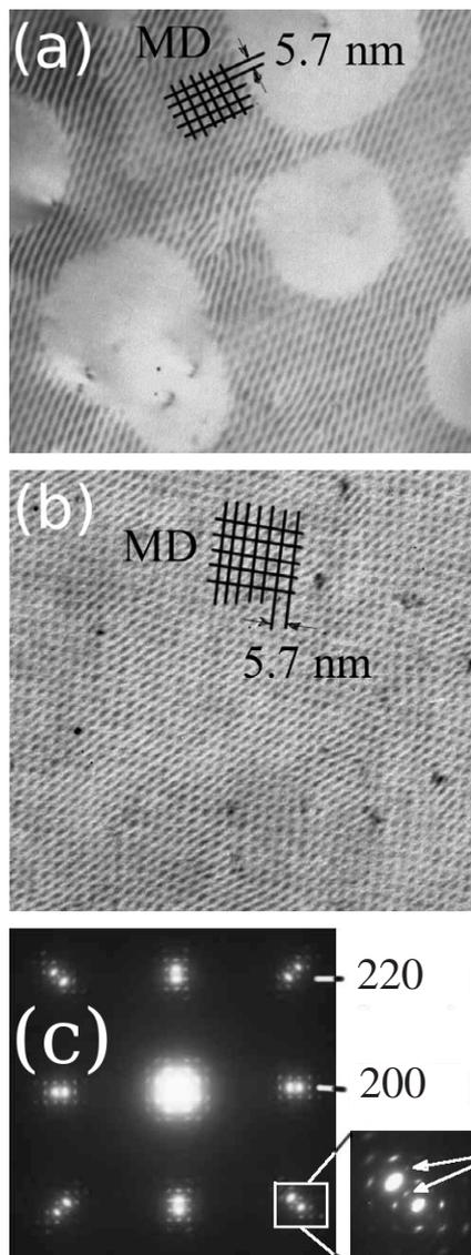
**Figure 8.** (a) Electron microscopy image of the Stransky–Krastanov mode of growth (island-like) of a thin PbTe layer on EuS; (b) electron microscopy image of the EuS–PbTe bilayer demonstrating the long range square misfit dislocation grid for the thicker, continuous, layers; (c) electron diffraction showing the satellites, accompanying the fundamental (200) and (220) reflections (see the arrows in the inset), arising from the periodic arrangement of dislocation lines at the interface.
