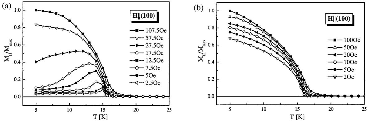
**Fig. 1.** The temperature dependence of magnetization of two PbS = 50 nm/EuS = 3 nm/PbS- $d$ /EuS = 3 nm structures on PbS(100) substrate with thin (Fig. 1a,  $d = 0.75$  nm) and thick (Fig. 1b,  $d = 5$  nm) PbS spacer.
