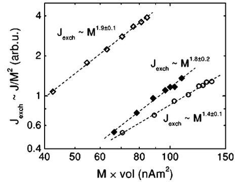
FIG. 6. Antiferromagnetic interlayer exchange coupling constant (coupling energy  $J$  divided by  $M^2$ ) plotted on a double logarithmic scale as a function of the saturation magnetization of the EuS layers for EuS(60 Å)/PbS(6 Å)/EuS(60 Å) (open diamonds), 60 Å/9 Å/60 Å (closed diamonds), and 40 Å/7.5 Å/40 Å (open circles) trilayers. Note the horizontal shift due to different sample areas.
