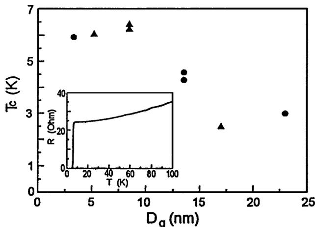
FIG. 3.  $T_c$  as a function of the dislocation grid period. Inset: resistance as a function of temperature for PbS/PbSe SL.
