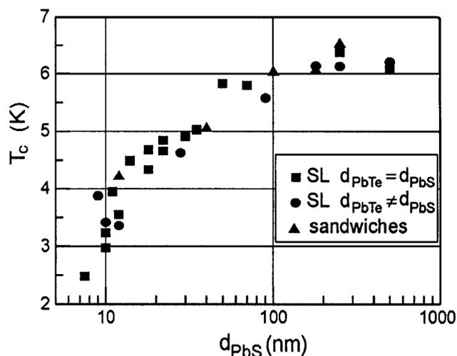
FIG. 1. Transition temperature as a function of  $d_{\text{PbS}}$  for PbTe/PbS layered samples.
