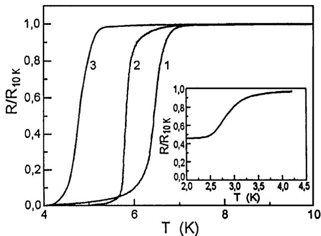
FIG. 2. Resistive transitions for semiconducting SLs and sandwiches. 1—PbS/YbS; 2—PbTe/YbS; 3—PbS/PbSe. Inset: resistive transition for PbTe/PbS SL with  $d_1 = d_2 = 7$  nm.
