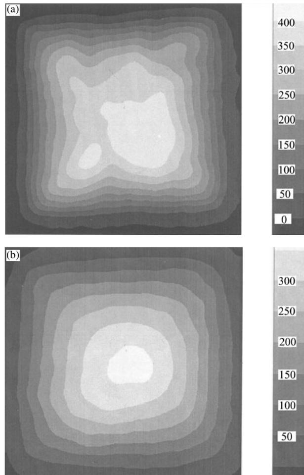
**Figure 5.** Distribution of the trapped magnetic flux for top (a) and bottom (b) planes.
