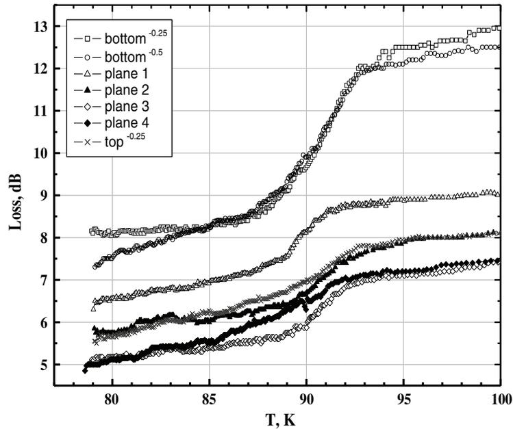
**Figure 2.** Temperature dependence of the microwave losses at planes 1–4, top plane polished by 0.25 mm ( $\text{top}^{-0.25}$ ), bottom plane polished by 0.25 mm ( $\text{bottom}^{-0.25}$ ) and bottom polished by 0.5 mm ( $\text{bottom}^{-0.5}$ ).
