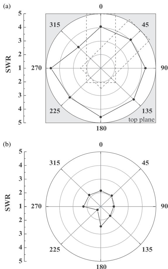
**Figure 6.** Dependence of the standing wave ratio (SWR) for the top (a) and bottom (b) planes on rotation angle of the waveguide window. Schematic positions of the measuring waveguide window on the sample surface for  $0^\circ$  and  $45^\circ$  are shown in (a) by dashed lines.
