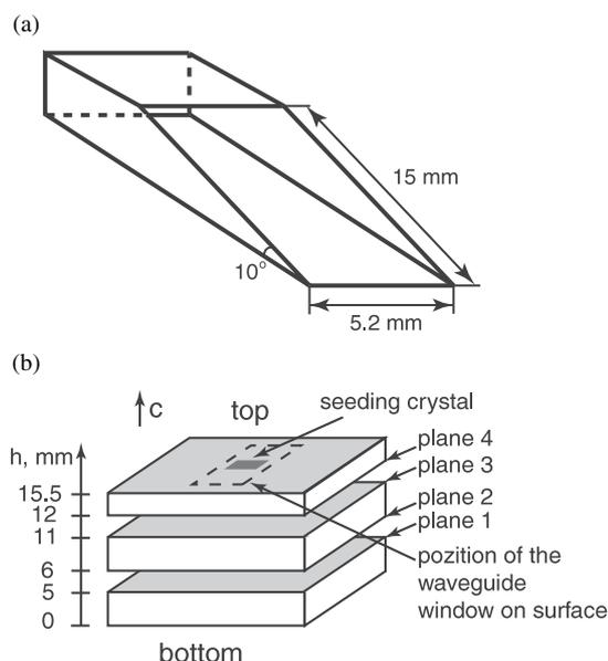
**Figure 1.** The measuring waveguide window (a) and the sample under study (b). The position of the waveguide measuring window on the sample surface is shown by the dashed line.
