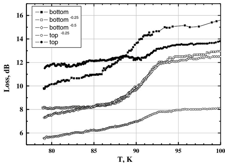
**Figure 3.** Temperature dependence of the microwave losses on the top non-polished plane (top), top plane polished by 0.25 mm, bottom non-polished plane (bottom), bottom plane polished by 0.25 mm ( $\text{bottom}^{-0.25}$ ) and bottom plane polished by 0.5 mm ( $\text{bottom}^{-0.5}$ ), showing degradation of the sample.
