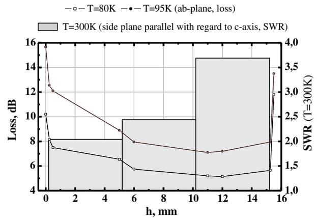
**Figure 4.** Dependence of the microwave losses in superconducting ( $T = 80$  K) and normal ( $T = 95$  K) states on distance from the bottom ( $ab$ -plane, lines), measured on the planes obtained by cutting the sample and comparison with SWR data at room temperature (in normal state on the side of the sample before cutting the sample) on the plane parallel to the  $c$ -axis ( $c$ -plane, bars) [2].
