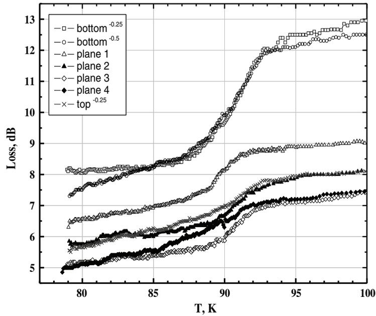
**Figure 2.** Temperature dependence of the microwave losses at planes 1–4, top plane polished by 0.25 mm ( $\text{top}^{-0.25}$ ), bottom plane polished by 0.25 mm ( $\text{bottom}^{-0.25}$ ) and bottom polished by 0.5 mm ( $\text{bottom}^{-0.5}$ ).
