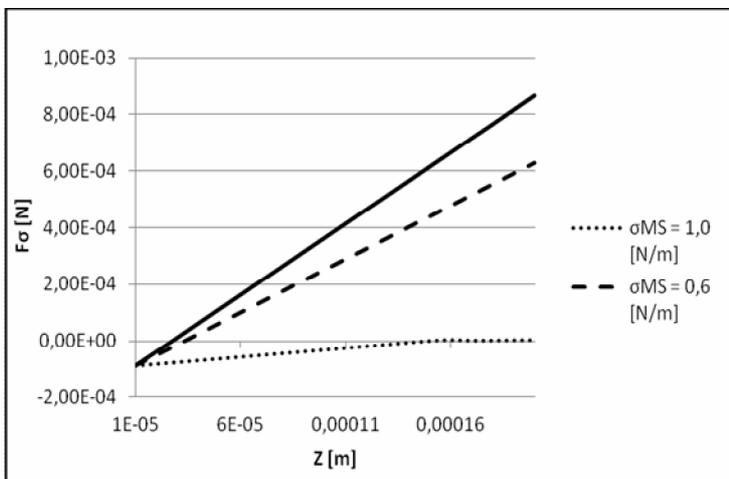
Fig. 1. Calculated capillary force  $F_c$  acting on inclusion particle of radius  $r = 0.00001 \text{ [m]}$  in the vicinity of interfaces for surface energy:  $\sigma_{\text{MS}} = 1.0 \text{ [N/m]}$ ,  $\sigma_{\text{MS}} = 0.8 \text{ [N/m]}$  and  $\sigma_{\text{MS}} = 0.6 \text{ [N/m]}$  against coordinate  $Z$ .
