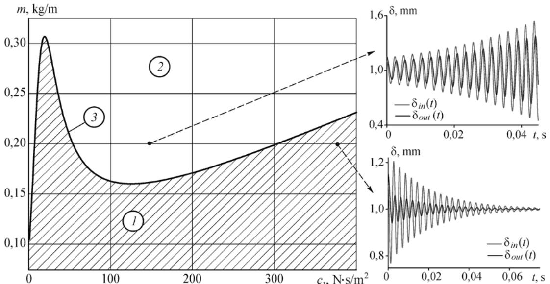
Fig. 3 Smooth seal stability region: 1 – safe operating area; 2 – unstable area; 3 – stability threshold
