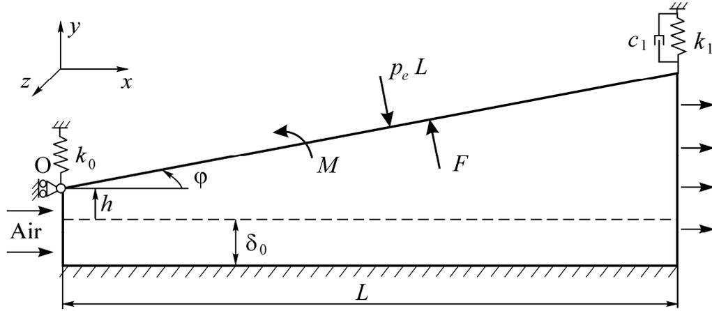
Fig. 2 Plane channel model with smooth walls
