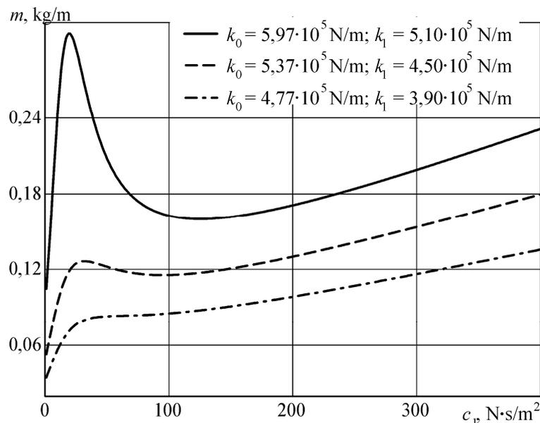
Fig. 6 Stability threshold for different stiffness
