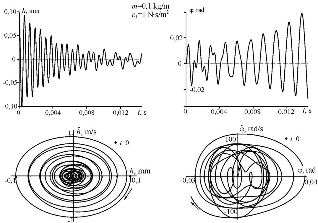
Fig. 9 Wall oscillations for different damping
