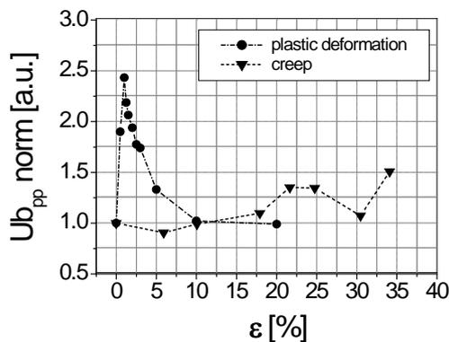
Fig. 8 Relation between the amplitudes of  $U_b$  envelopes and prior deformation due to plastic flow (circles) and creep (triangles)
