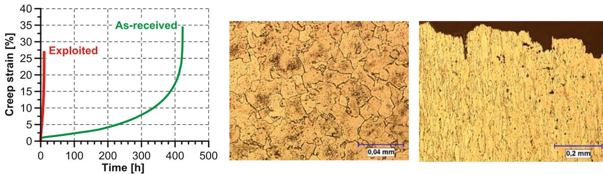
Fig. 1 Comparison of tensile creep curves ( $\sigma=230$  MPa,  $T= 773$ K) for the 13HMF steel in the as-received state and after exploitation by a period of 144000 h (a), and its metallographic structures for the initial state (b) and after 144000 h of work (c)
