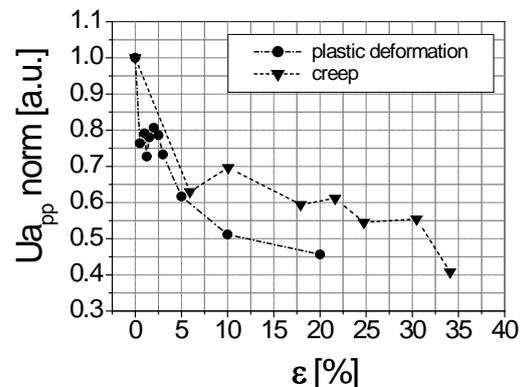
Fig. 9 Relation between amplitudes of  $U_a$  envelopes and prior deformation due to plastic flow (circles) and creep (triangles)
