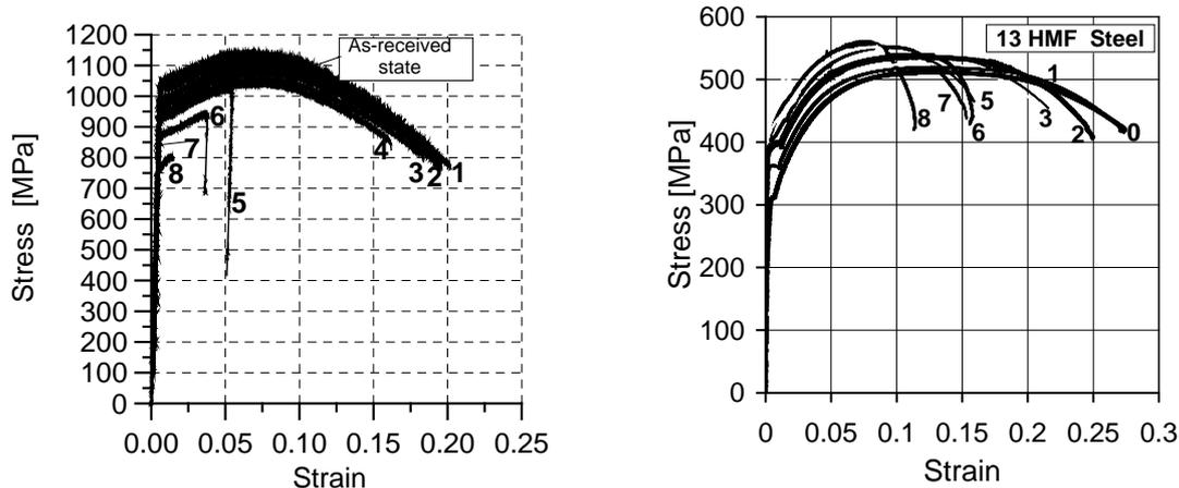
Fig. 2 Tension characteristics of: (a) the 40HNMA steel after creep for 100h (1), 241h (2), 360h (3), 452h (4), 550h (5), 792h (6), 929h (7) and 988h (8), and (b) the 13HMF steel after creep for 149h (1), 300h (2), 360h (3), 407h (4), 441h (5), 587h (6), 664h (7), 796h (8) and 1720h (9)
