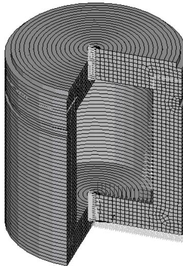
Fig. 3 Finite element model of the container
