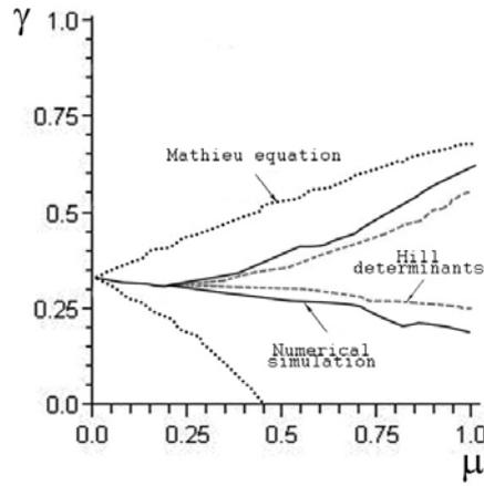
Fig.6. Boundaries of the stability/instability regions of the longitudinal vibrations.
