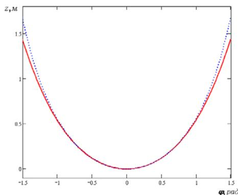
Fig.4. Trajectory of mode of coupled vibrations in configuration space. Entire line represents the analytical solution; point line represents the checking numerical calculation.
