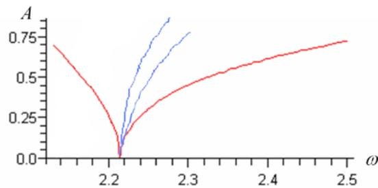
Fig.9. Boundaries of the stability/instability regions of the non-localized mode of the system (3)
