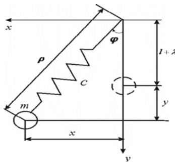
Fig. 1. The spring pendulum
