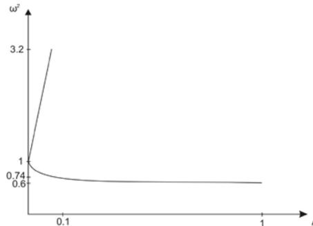
Fig.7. Boundaries of the stability/instability regions for mode of coupled vibrations.
