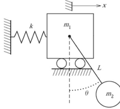
Fig. 2. The two-DOF system containing the pendulum as absorber.
