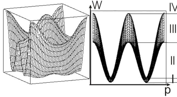
Fig. 1. The potential relief  $W_p$  in a quadrupolar molecular chain. (left) 3D image. (right) View along a valley. (I) Ordered phase. (II) Phase of correlated movements when  $p$  is finite,  $m$  is infinite. (III) Phase of correlated movements when both  $p$  and  $m$  are infinite. (IV) Completely disordered phase.
