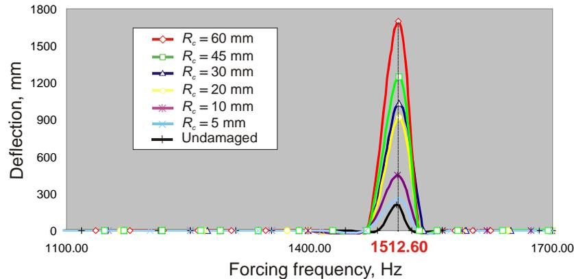
Fig. 3. Harmonic deflection responses vs radius of impacted site.
