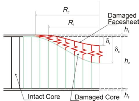
Fig. 1. Impact-damaged region.
