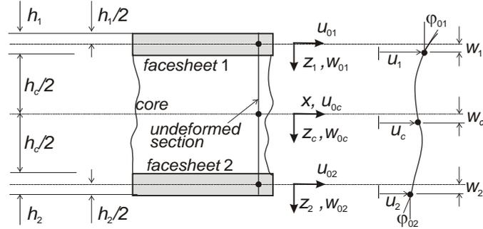
Fig. 2. Sandwich plate cross-section.
