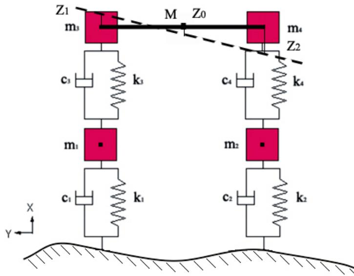
*Fig. 4 The oscillation model*
