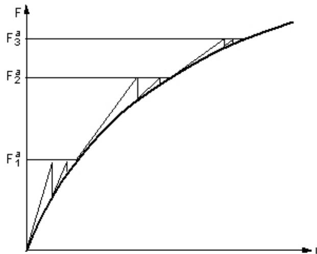
Fig. 1 Approximation of Newton – Raphson procedure
