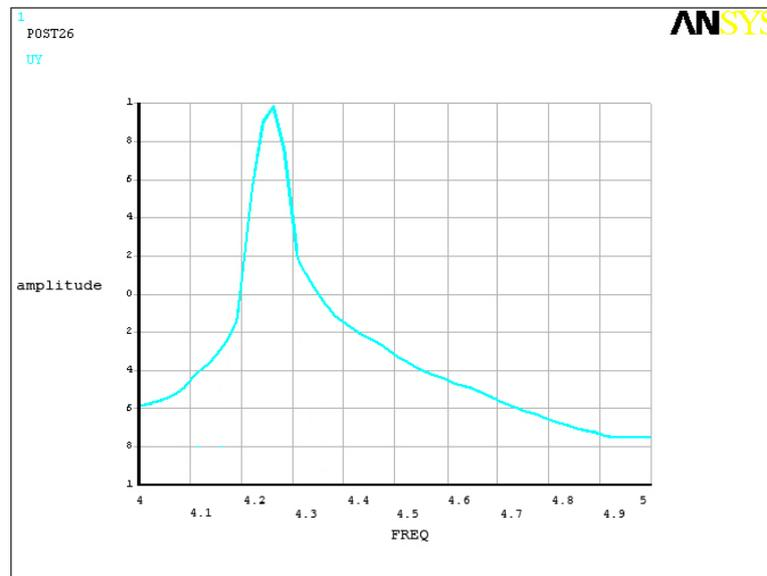
Fig. 6 Gain-frequency characteristic of nonlinear oscillation
