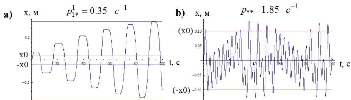
$$m = 500 \text{ kg}; \quad F_0 = 100 \text{ H}; \quad 2 \cdot F_* / F_0 = 2; \quad |x_0| = 0.1 \text{ m}$$
