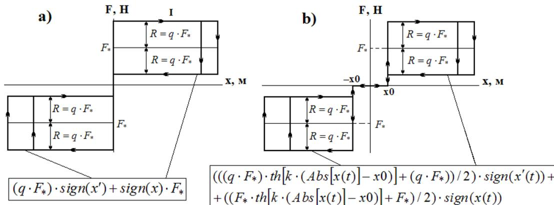
**Fig. 1 Force characteristics with loops of hysteresis**
