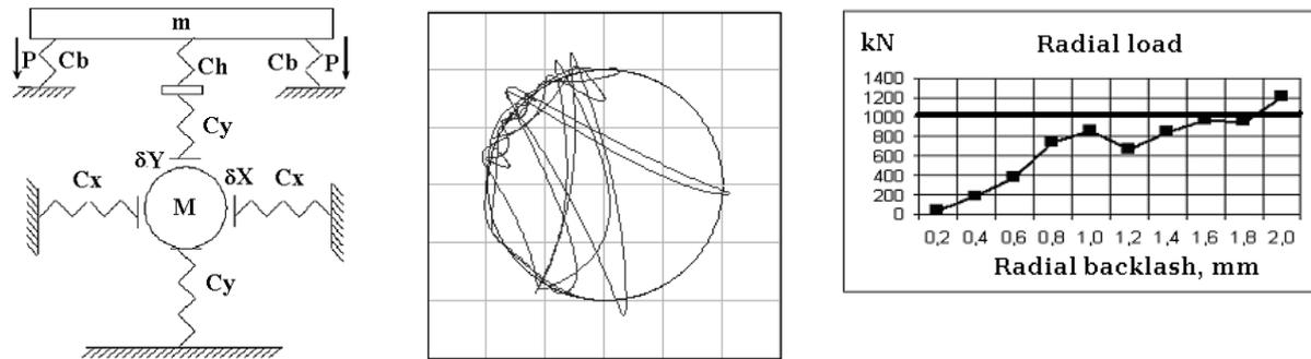
Fig. 8 Calculation scheme of shaft-bearing-housing nonlinear system, shaft motion trajectory and maximal radial loads on bearing
