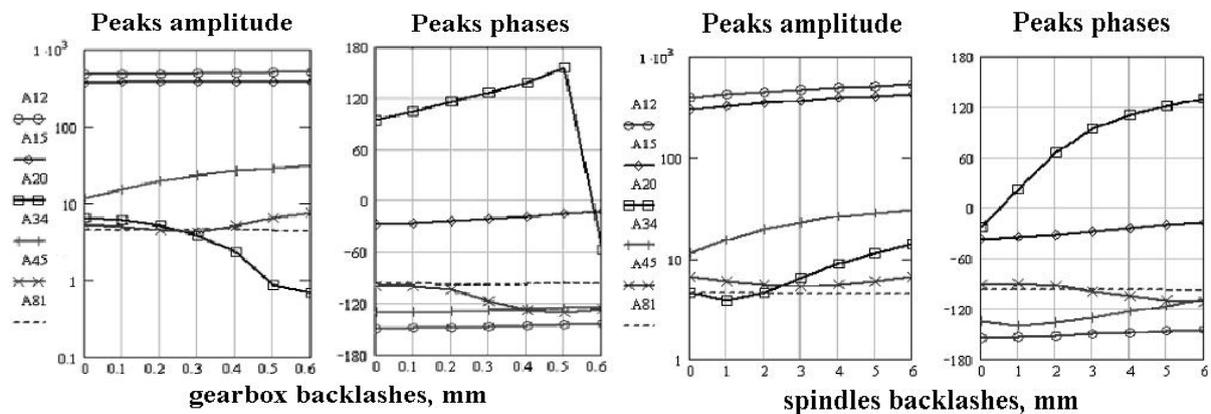
Fig. 7 Variation of the torsional natural frequencies and phases due to backlashes in the gearbox and spindles
