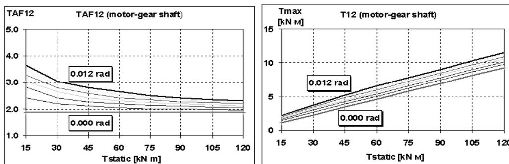
Fig. 3 Static torque influence on TAF and peak torque  $T_{max}$  in motor shaft (C12) (Simulation)
