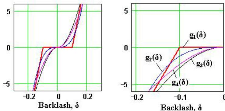
Fig. 5 Non-smooth stiffness characteristic approximation with continuous functions
