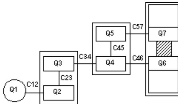
Fig. 2 The multi-body calculation scheme of the hot rolling mill (one stand)
