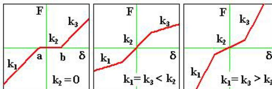
Fig. 1 Piecewise linear non-smooth stiffness characteristics in the rolling mills
