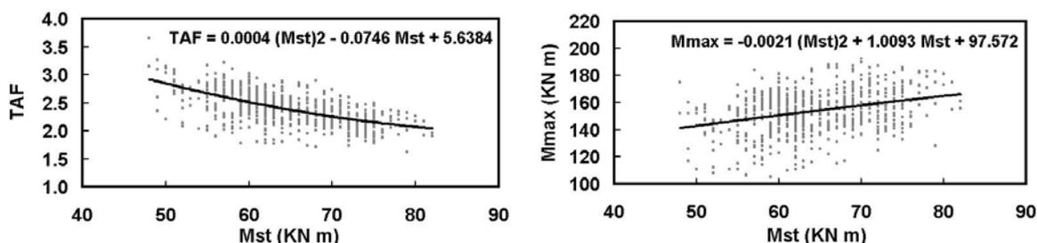
Fig. 4 Static torque influence on TAF and peak torque  $M_{max}$  in motor shaft (C12) (Telemetry measurements with the strain gauges)
