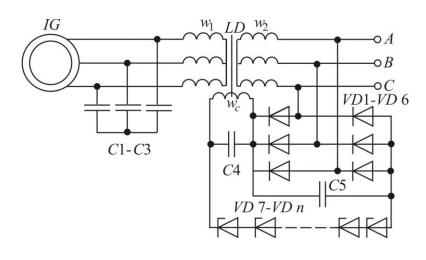
For wide using induction generators (*IG*) in isolated power plants it is necessary means of voltage and frequency stabilization. One of the possible circuits for solving such problem is presented on the figure.
