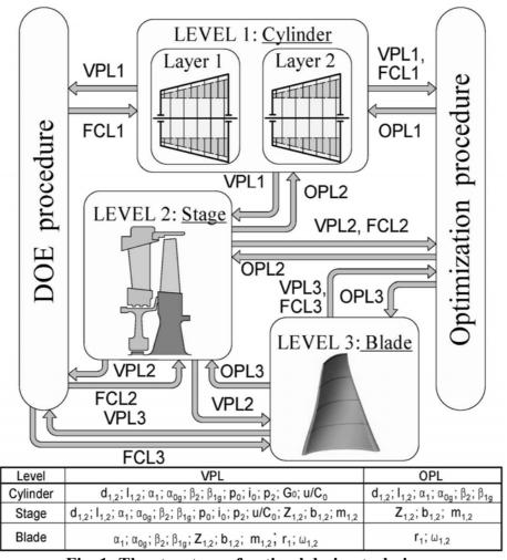
Fig. 1: The structure of optimal design technique
