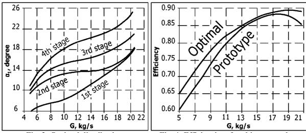
Fig. 3: Optimal distribution of angles α<sub>1</sub> along the flow path subject to mass flow
