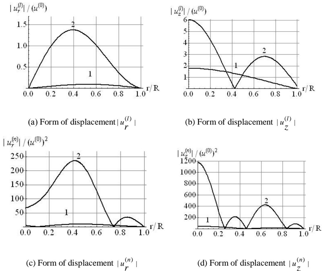
*Fig.1 – Amplitude forms of displacement in first linear and second nonlinear harmonics for the longitudinal-shear waves with  $\lambda = 10R$  in a cylinder with fixed boundary.*
