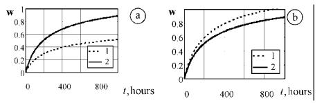
Fig. 3 Binder rupture life exhaustion  $w^1$  (1),  $w^2$  (2) for  $c_* = 0.002$  (a) and  $c_* = 0.001$  (b)
