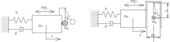
a) single-impact absorber model b) double impacts absorber model Fig.4. Model of the pendulum impact absorber.
