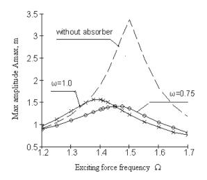
Fig.7. Maximal amplitude Amax in relation to exiting force frequencies  $\Omega$  for single impact pendulum absorber ( $\mu$ =0.04, r=0.6).
