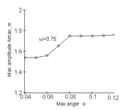
Fig. 10. Maximal amplitude Amax depending on pendulum clearance angle  $\alpha$  ( $\mu$ =0.04, r=0.6) for multi-impact absorber shown in Fig.4b.
