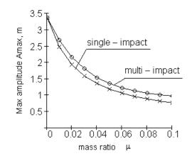
Fig.8. Maximal amplitude depending on  $\mu$  –ratio for single-impact absorber ( $\omega$ =0.75, r=0.6) and multi-impact absorber ( $\omega$ =0.75, r=0.6,  $\alpha$ =0.05) and  $\Omega$ =1.5 for both case.
