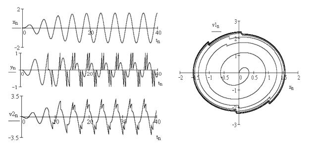
Fig. 12. Plots of dependence of motion parameters on time: x=x(t), y=y(t),  $v_2r=v_2r(t)$  and phase map for classical impact absorber in case of:  $\Omega=1.5$ ,  $\lambda=1.5$ , c=1,  $\mu=0.04$ , r=0.6.
