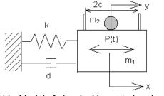
Fig.11. Model of classical impact absorber.
