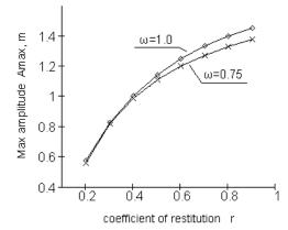
Fig.9. Maximal amplitude Amax in relation to coefficient of restitution r for single impact pendulum absorber ( $\mu$ =0.04, r=0.6).
