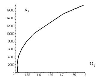
Fig.2 The backbone curves of two conjugate modes
