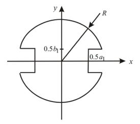
Fig.1 Circular plate with two cutouts
