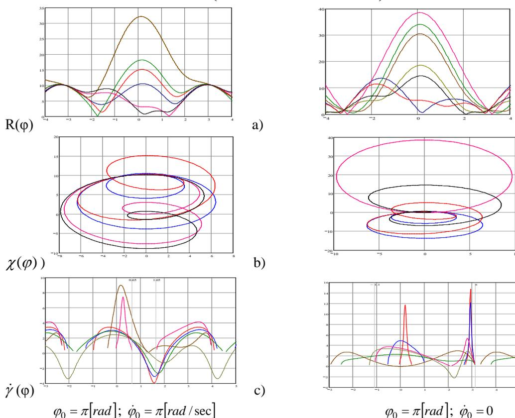
Fig. 5. Vector rotator of the heavy gyro rotor: a) the intensity portrait; b) the hodograph; c) the angular velocity for different values of angle  $\beta$  and for different initial conditions
