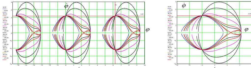
Fig. 4. Transformation of a phase trajectory presentation of the heavy gyro-rotor with rotating axis that are without intersection for different values of normal distance between axes and for a corresponding initial condition.
