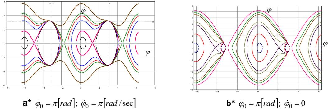
Fig. 3. Transformation of a phase trajectory of the heavy gyro rotor with rotating axis that are without intersection for different values of disk inclination angle  $\beta$  to the axis of self rotation and for two different initial conditions:
