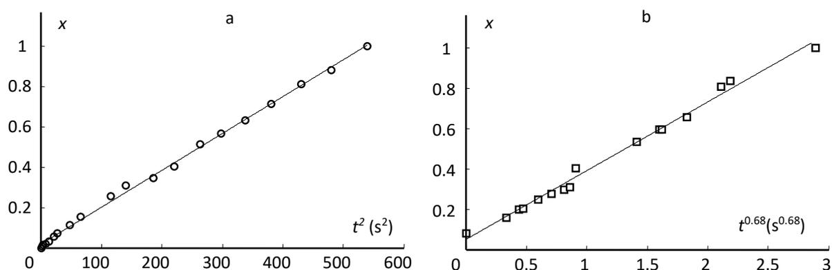
FIG. 1. Time dependence of the fraction crystallized for polymorphous (a) and for secondary (b) crystallization of amorphous films of  $Sb_2S_3$
