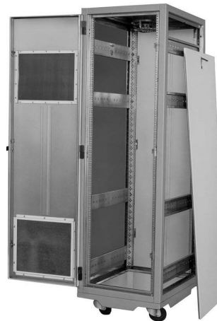
Fig. 8. Control cabinet with upgraded protection against EMP equipped with special loops, conductive rubber gasket, special coupling and connecting elements, shielded air vent windows, etc. (Equipto Electronics Corp.)
