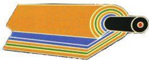
Fig. 12. Multilayered shielding of poly-sandwich developed by Belden
