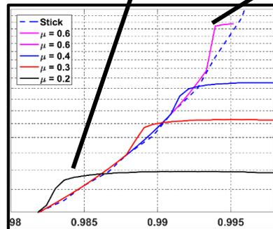
$\mu = 0.6$  : big amplitude of normal forces for excitat. frequencies close to resonance
