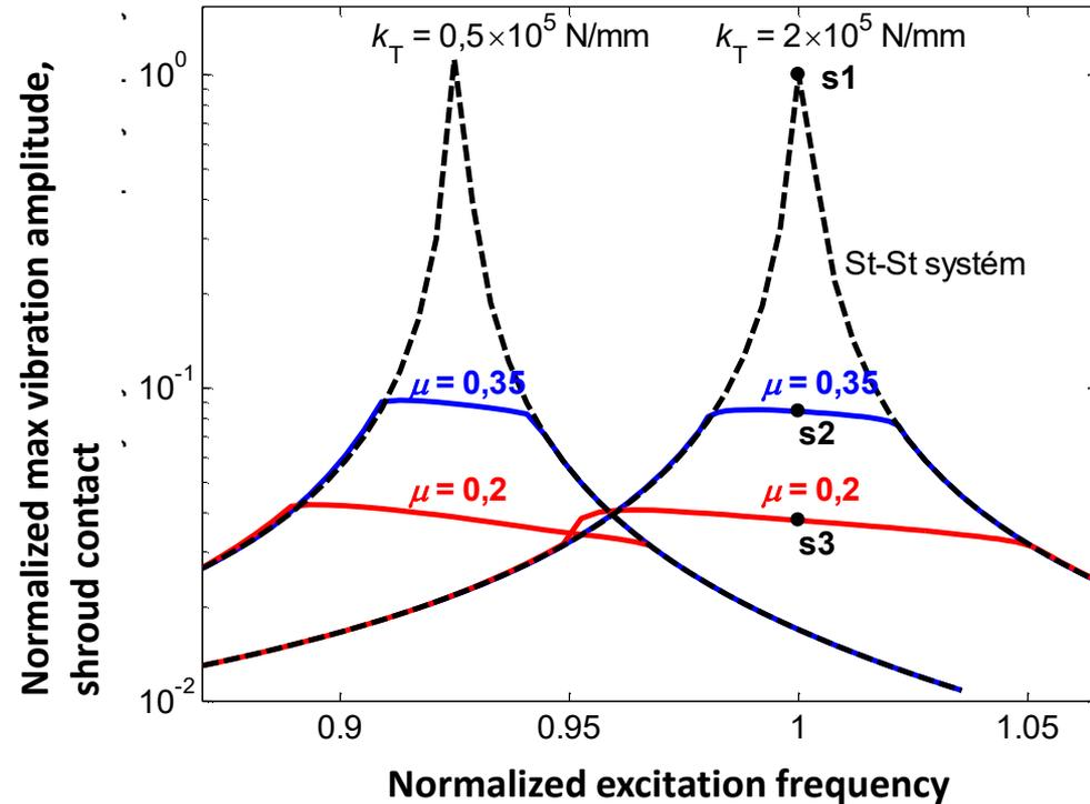
Limited number (10) of mode shapes for approximation of blade dynamic behavior → necessity to fit contact stiffnesses (influencing resonant frequencies of computational model)
