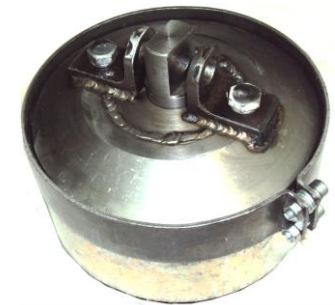
Bistable actuator with ferromagnetic shunt
