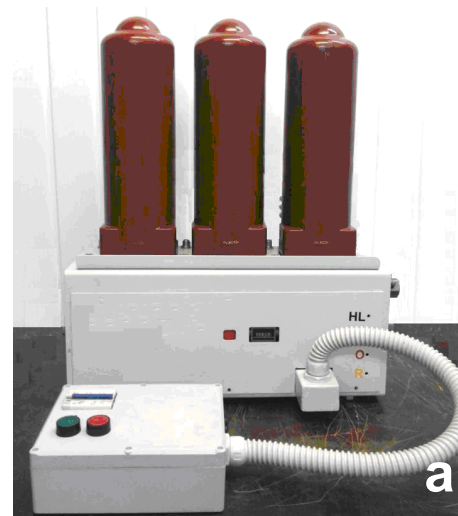
Prototypes of circuit breaker (a) and contactor (b) with microprocessor control systems
