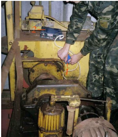
Magnet-coercive testing of a crane's metalwork and crane wheel
