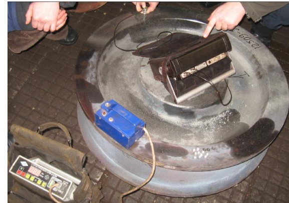
Magnet-coercive testing of a crane's metalwork and crane wheel
