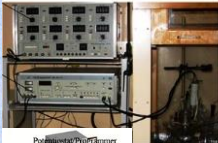
Setup for electrochemical deposition
