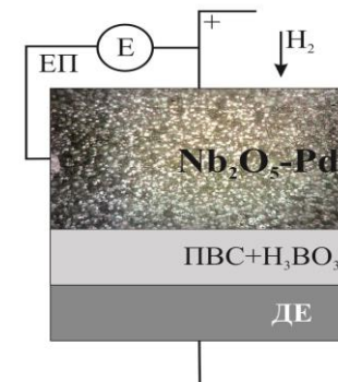
Scheme of the indicator electrode of the sensor system for the detection of hydrogen
