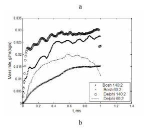
Fig. 2. Mass rate for Delphi and Bosch injectors; ambient pressure 2 MPa; a – injection pressure 140 MPa and 160 MPa; b – injection pressure 60 MPa and 140 MPa
