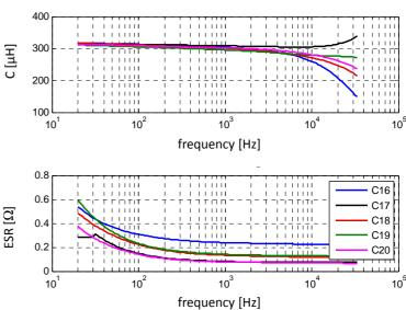
Fig. 3. Small signal measurement of some of the aluminum based electrolytic capacities.
