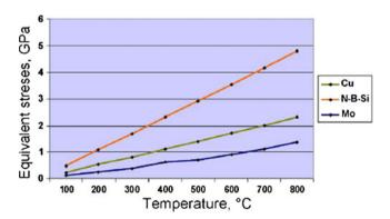
Fig. 5 Dynamics of stress rise in system "grain-metal phase-coatingbond" with diamond grain AC 100; width of coating 15  $\mu$ m
