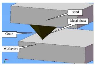
Fig. 6 3D model "bond-grain-metal phase-workpiece" with finite-element mesh
