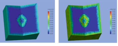
obtained results were compared. The influence of the availability of coatings on diamond grains is studied and the coating composition, allowing reduction of equivalent stress in the grain, is defined [12].
